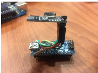
nRF24L01 transceiver module with Arduino Nano
